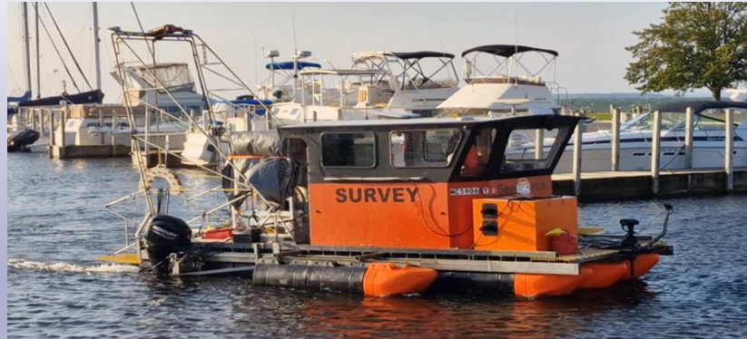
GeoSearch laden with 1200kg winch during sea trials
