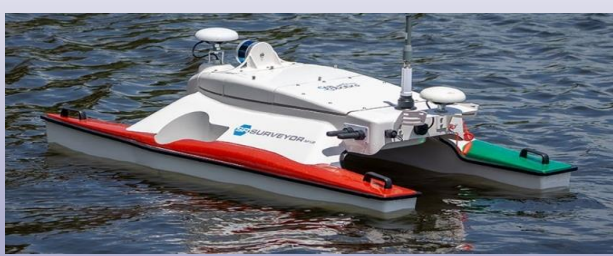
Automated Surfaced Vessel
